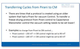
I've seen people who have actually transferred from a Pirani system to a steam sterilizable freeze dryer, and the process would not work because the new pressure was higher than it should have been because it was using a Capacitance Manometer. I'm going to show you that in a second as well. Another one, if we were controlling at 100 millitorr with the Pirani, we might set the Capacitance Manometer to 60
