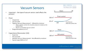
although you're not going to see it when you're looking at Pirani control because it's not changing. The true vacuum in the system actually increases through the process. This could be a problem, because if you're going to transfer this cycle from your older freeze dryer to either a new freeze dryer or a production freeze dryer, it will not transfer properly because the new system's going to be using a Capacitance Manometer.
