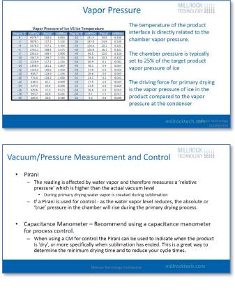
water vapor. So, if you're using these for control, the true vacuum in the system is going to change throughout the process as the water vapor content changes, and water vapor content reduces during
