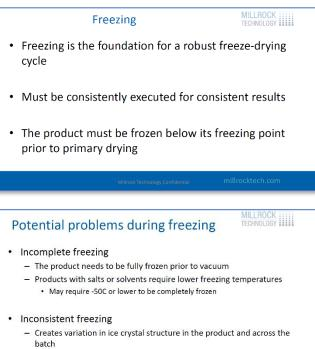
freeze, and it's important to understand that all of your product is frozen. Inconsistent freezing is another problem. Inconsistent freezing can create variations in ice crystal structure in the product and across the batch, which results in variation to the process.
