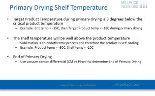
we're driving energy into the process... Sublimation is an endothermic reaction, so the product is actually going to be cooler than the shelf during sublimation.
