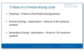
down to the three to 5% moisture content range. This may or may not be sufficient dryness for your product. In some cases, you need a secondary drying cycle, it's called desorption. And the temperature of the shelf has increased. And this can be used to dry the product to less than 1% moisture. Be aware that there are some products that can be too dry, and it affects their efficacy once the freeze-drying process is done.
