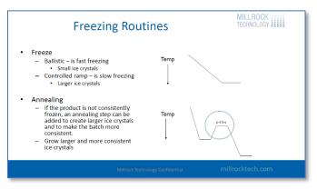
annealing step where we have a ramp rate down to a temperature hold for a period of time, raise the temperature of the product to let's say -20, -15, hold it for a period of time, and then freeze it again before we go into primary drying. This is going to grow larger ice crystals, and it's going to make them more consistent.
