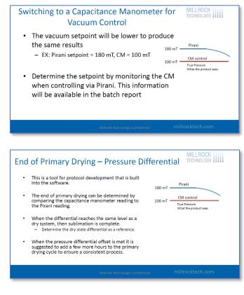
Capacitance Manometer in a dry state, and once that reaches the differential, let's say it's five millitorr just as an example, then what we suggest is that's the end of primary drying. You just add a few more hours of hold at the existing pressure and temperature to verify that everything in the system has reached its dry state, and then you can move on to secondary drying.
