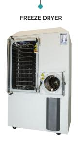
The freeze dryer is designed to accommodate LyoBead specific application requirements including pre-frozen shelves for storage of the frozen beads prior to freeze drying.
