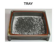
An aluminum tray with anodized finish enables bead production and collection, transfer, freeze drying process, and postfreeze drying storage.
