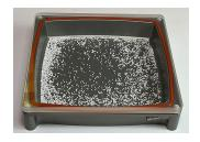
An aluminum tray with anodized finish enables bead production and collection, transfer, freeze drying process, and post-freeze drying storage.
