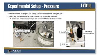
directly mounted on it along with an RTD, which you can see in the bottom right here.
