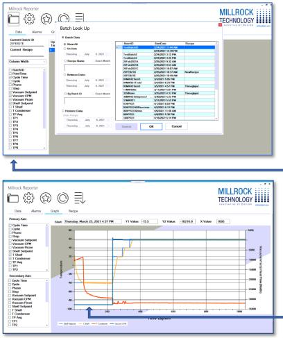
Data is collected and stored for all process parameters, both set points and read outs, in the freeze drying cycle. Millrock Reporter lets you pick and choose which parameters you want to see and will provide the information in either an alpha-
