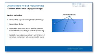
Starting with the freezing challenges, we can start with random nucleation. With bulk trays, this is typically a problem with liquid fills. It's not typically a problem with, for example, tissue applications or such. Random nucleation is when multiple nucleation sites occur within a tray. What this causes, usually, is an inconsistent crystallization in crystal growth within the tray, which would lead to a different size
