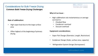
capacity due to large surface area of the product, which leads to a high rate of sublimation that could lead to issues or at least challenges down the road. So, with the rate of sublimation, with that surface area being very high includes many of the applications. API and tissue are especially important here. At the very beginning of primary drying, we could see a much higher rate of sublimation, and that could lead to issues such as choked flow, condenser overload, and condenser bypass.
