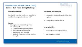
temperature because the refrigeration system doesn't have the capacity. The temperature starts to go up, and you could hit the condenser overload conditions quickly. Refrigeration issues sometimes could cause that. It is important to follow through your maintenance programs and preventative maintenance programs to prevent any refrigeration system problems prior to them happening.
