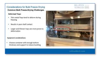
top tray and the bottom tray here with the gap between the tray and the shelf. This can result in poor shelf contact, which leads to poor heat transfer in primary drying, and further problems down the road. Typically, a larger tray is more prone to deformation than a smaller tray, and a thinner tray is more prone to the formation than a thicker tray. So, it is important to choose your container with enough bottom thickness and support material to reduce buckling and deformation.
