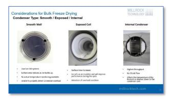
first is the smooth wall condenser. These were used on old systems. They're not very popular these days. They have their own issues. For example, the surface area reduces as ice builds up. The ice deposits on the wall of the condenser.
