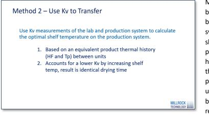
Method two for cycle transfer would be to use the Kv measurements between the lab and production system to then calculate the optimal shelf temperature on your production system. This is based on having an equivalent product thermal history, both heat flux and product temperature between the units and it accounts for a lower Kv by increasing the shelf temperature resulting in an identical drying time.
