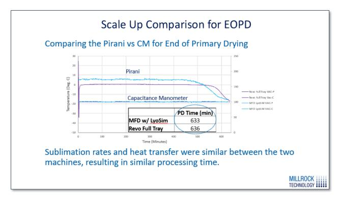
An extra piece of data here shows the primary drying time between these two cycles, the MicroFD at OC and the REVO at 4C, was within about three minutes of each other. The sublimation rates and heat transfer were very similar between the two units resulting in similar drying times.
