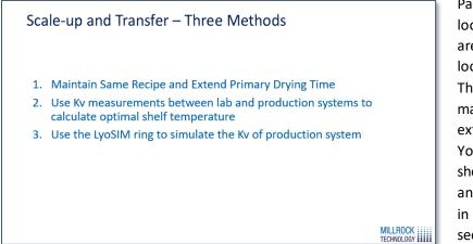
Past freezing, when we are looking at primary drying, there are three main methods that we look at for transferring the cycle. The first and simple method is to maintain the same recipe and extend the primary drying time. You're going to keep the same shelf temperature and pressure and extend primary drying time in your production system. The second would be to use Kv measurements between the lab
