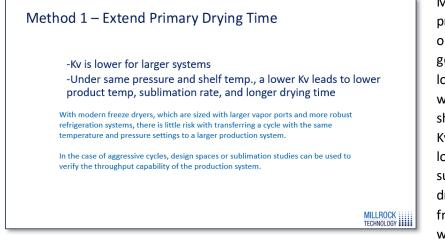
Method one, extending primary drying time, is based on the observation that Kv is generally across the board lower for larger systems. So with the same pressure and shelf temperature, the lower Kv in a larger system leads to a lower product temp, sublimation rate, and longer drying time. With modern freeze dryers which are sized with larger vapor ports and
