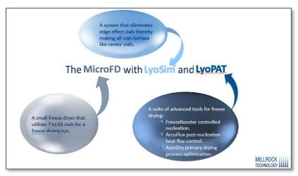
Using a larger tray style unit and simply putting a small array of vials in the center of the tray will not effectively help protocol development, because the vials will not dry or behave representative of a full batch of vials in that system.
