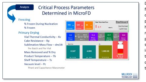
During the cycle is the first time we measure our critical process parameters. Again, the heat flux can be used to measure all of the process parameters we see here, most importantly the vial thermal conductivity, the cake resistance as well as the mass flow.
