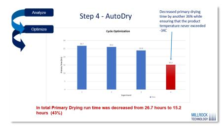
And then the overall results for that show that we were able to overall reduce our primary drying time by 43%. But again, I'll reiterate that much of this optimization did not occur in primary drying, but occurred in freezing to start. We had to lay optimized foundation within our batch in our frozen state before we can fully optimize in primary drying.
