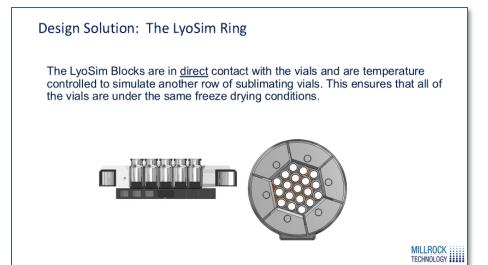
Here we can see an actual picture of what this array looks like with the vials and the Ring around the outside and we can see some data that was taken gravimetrically about 25% of the way to primary drying where we record very good uniformity across the batch and do not see any pronounced edge effects
