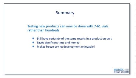
In summary, those three methods of transfer were one, to keep the same product temperature or keep the same shelf temperature and pressure and extend the primary drying time on your production unit, two, to compare the Kvs between your lab and production unit and use those to calculate an adjusted shelf temperature on your production unit, or three, to use the MicroFD
