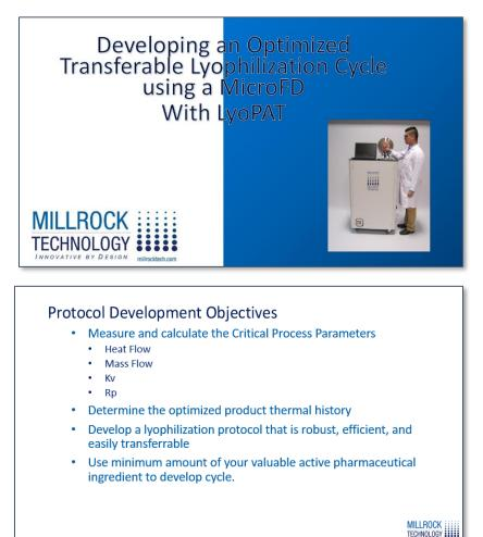
Some of the main protocol development objectives that are critical during the process of developing your cycle are to measure and calculate your critical process parameters, including heat flow, mass flow, the vial heat transfer coefficient (Kv), and the product cake resistance (Rp).
