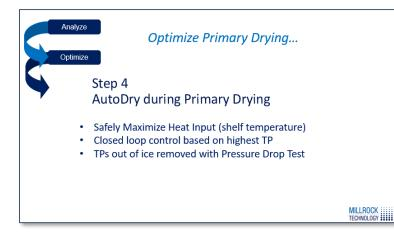
This is where AutoDry comes into play. AutoDry safely maximizes your shelf temperature and your heat input while keeping your product safely below its critical temperature based on closed loop control looking at the highest thermocouple in the batch. It also monitors the thermocouples as it is drying to determine when they are pulled out of ice with a pressure drop test.
