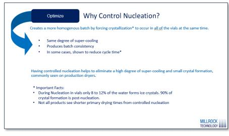
In some cases, using controlled nucleation can be shown to reduce cycle time but it's important to note that that is not the primary benefit of controlled nucleation. The primary benefit of controlled nucleation is to create uniformity across the batch and consistency between batches, so you always have the same degree of super cooling.
