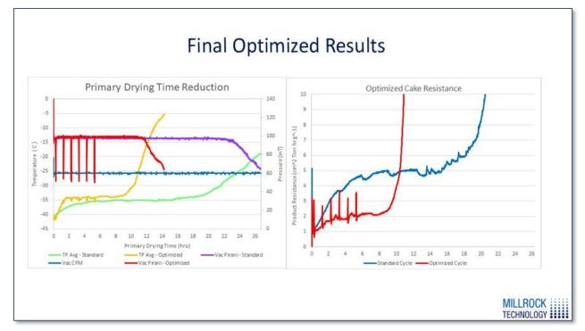
Here we can look at our final optimized results and we see our product temperature and pressure convergence for the initial run in the optimized run. We can see that our product temperature while higher than the initial run was still safely below our critical temperature and we can see we have also significantly reduced our cake resistance through this optimization process.
