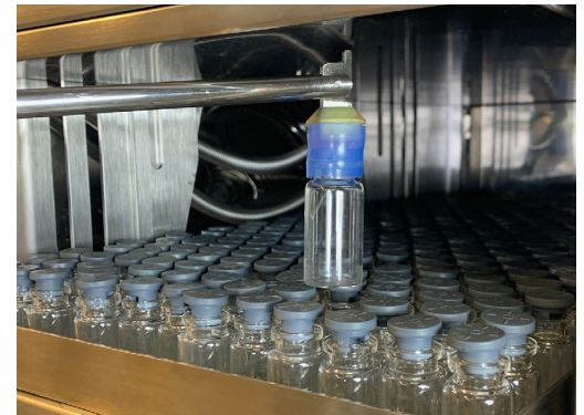
Spider L/XL grabber shown with caged support for maximum grip (100ml serum vials shown)
