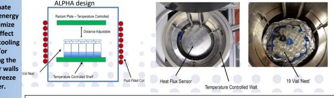
Made controlled temperature walls. Also tried adding commercial insulation and aluminum shield to minimize edge effect.
