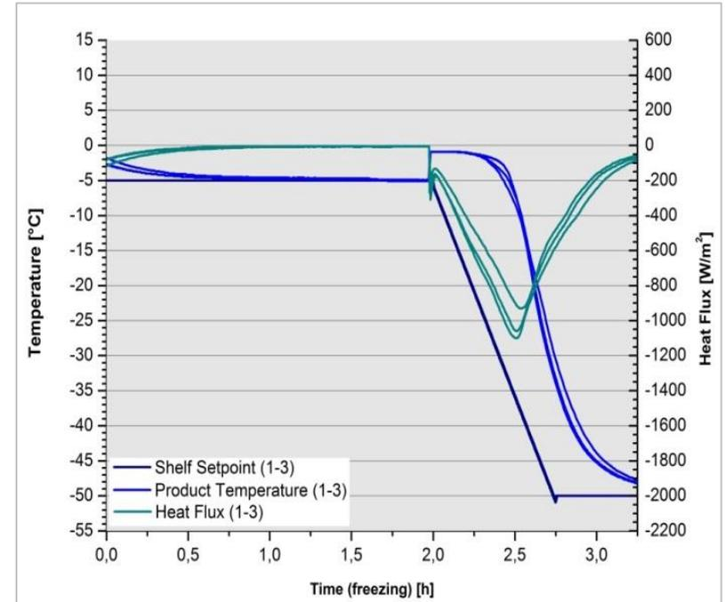
Heat flux sensor can reliably indicate nucleation events
