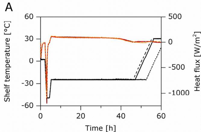
➤ No apparent impact of degree of shelf loading on heat flux measurements.
